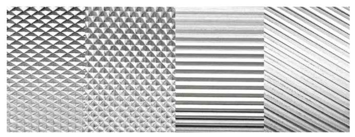
The knurling quality and the tool life can be improved substantially by optimising the knurling by changing the rough-turn diameter and/or the pitch.
