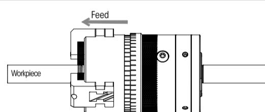
Fig. 5: Feed in Z direction
